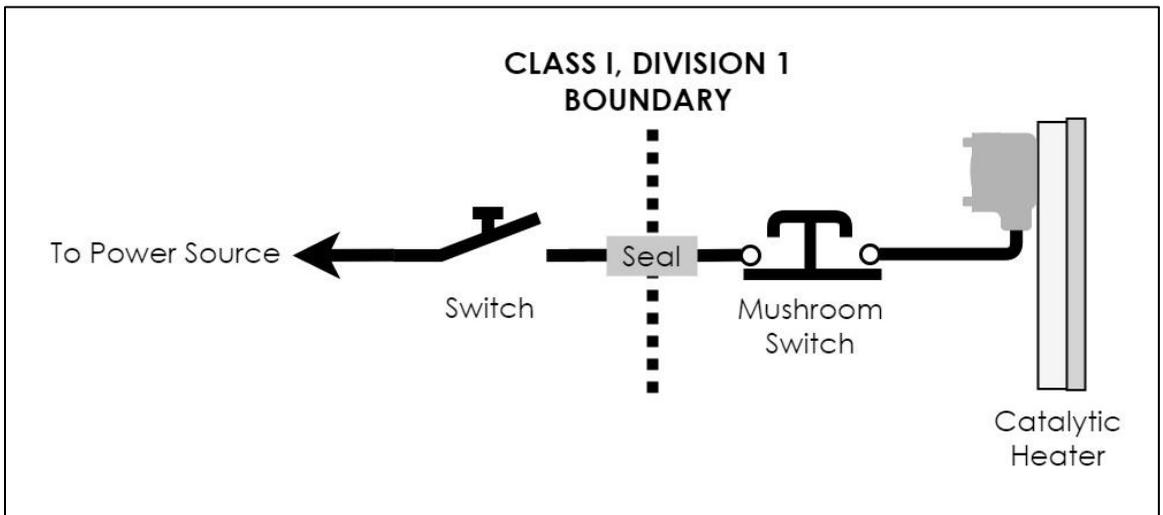
**Figure 4.** Typical Class I, Division 1 installation.
