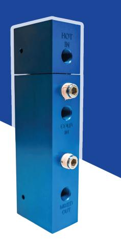
The Steady Heat Controller prevents instrumentation overheating by blending heated natural gas from an Instrument Gas Heater with ambient temperature natural gas to deliver temperature-regulated gas.
